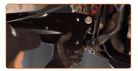
Tighten the fasteners connecting the control arm to the rear knuckle. Use a drive socket #18. Use a torque wrench. Tighten it to 90 Nm torque.+90°
