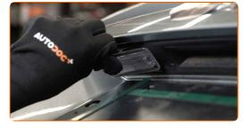
Screw in the fastener of the number plate light housing. Use a Phillips screwdriver.
