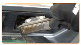
Treat the connectors of the number plate light. Use dielectric grease. Use a flat screwdriver.
