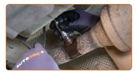
Tighten the oxygen sensor fastener. Use a flare nut spanner #22. Use a torque wrench. Tighten it to 37 Nm torque.
