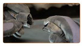
Clean the oxygen sensor fastener. Use a wire brush. Use WD-40 spray.
