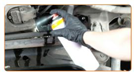
Detach the oil filter from the filter cover.
