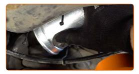
Attach the fuel filter fasteners. Use nippers.
