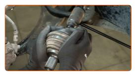
19 Attach the CV joint puller.
