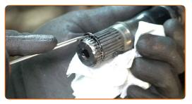
Clean the splines of the drive shaft CV joint. Use a wire brush. Use all-purpose cleaning spray.
