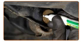
Unscrew the arm fastening to the beam. Use a combination spanner #18. Use a drive socket #18. Use a ratchet wrench.
