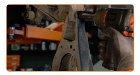
Remove the fastening bolt.
