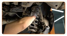
Unscrew the fastener connecting the control arm to the rear knuckle. Use a combination spanner #18. Use a drive socket #18. Use a ratchet wrench.
