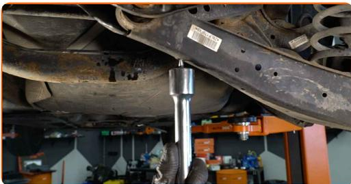
**10** Loosen the fastener that connects the control arm to the rear knuckle. Use a combination spanner #18. Use a drive socket #18. Use a ratchet wrench.
