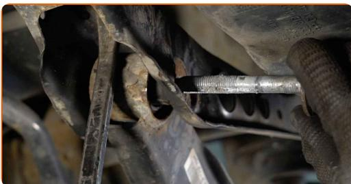
**12** Remove the support from under the arm.
