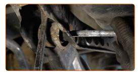
Remove the support from under the arm.
