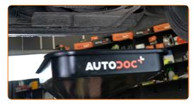
Clean the area of the oil pan drainage hole. Use a nylon cleaning brush. Use all-purpose cleaning spray.
