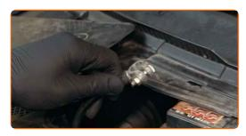
Loosen the alternator fasteners. Use HEX No.H8.
