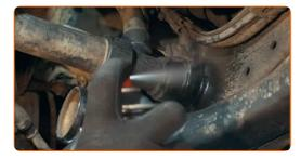
Disconnect the coolant pipe retaining clip.
