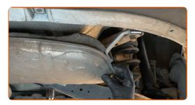
Remove the fastening bolt.
