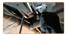
Unscrew the fastener connecting the control arm to the rear knuckle. Use a combination spanner #18. Use a drive socket #18. Use a ratchet wrench.
