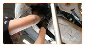
Tighten the fastener connecting the control arm to the rear subframe. Use a combination spanner #18. Use a drive socket #18. Use a torque wrench. Tighten it to 95 Nm torque.
