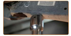
Unscrew the arm fastening to the beam. Use a combination spanner #18.
