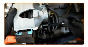
Replacement: brake caliper – AUDI A3 Hatchback (8P1). Tip from AUTODOC:
