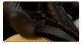
Reinstall the air filter cover. Fasten it.
