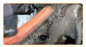
Clean the splines of the drive shaft CV joint. Use a wire brush. Use WD-40 spray.
