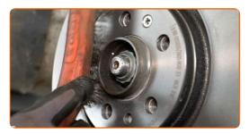
Unscrew the brake disc fasteners. Use a Phillips screwdriver.
