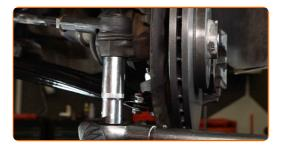
Tighten the lower fasteners of the suspension strut. Use a drive socket #18. Use a torque wrench. Tighten it to 50 Nm torque.+90°
