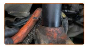
Unscrew the lower fastener connecting the shock strut to the steering knuckle. Use a drive socket #18. Use a combination spanner #18. Use a ratchet wrench.
