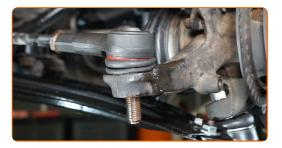
Screw on the fastening nut that connects the tie rod end to the steering knuckle. Use a drive socket #19. Use a ratchet wrench.
