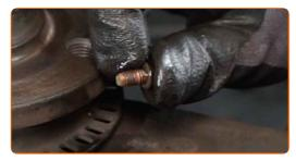
Remove the brake disc cover.
