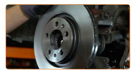
Unscrew the fastener connecting the drive shaft to the wheel hub. Use a drive socket #30. Use a ratchet wrench.
