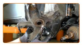
Clean the fasteners of the brake disc cover. Use a wire brush. Use WD-40 spray.
