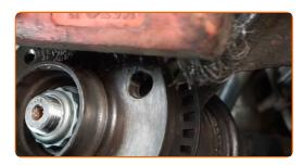
Treat the contacting surface. Use ceramic grease.
