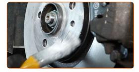
Clean the brake disk surface. Use a brake cleaner.
