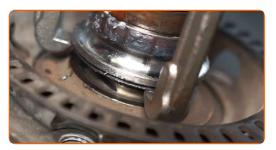
Clean the wheel hub mounting seat. Use a wire brush. Use WD-40 spray.
