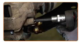
12 Remove the brake caliper.
