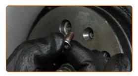
16 Remove the brake disc.
