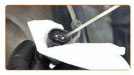
68 Attach the ABS sensor connector.
