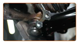
Detach the driveshaft from the steering knuckle.
