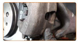
78 Tighten the brake caliper fasteners. Use HEX No.H7. Use a torque wrench. Tighten it to 28 Nm torque.
