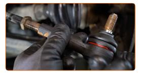
Replacement: track rod end – AUDI A3 Hatchback (8L1). Tip from AUTODOC:
