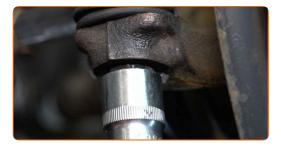
Tighten the fastening nut connecting the tie rod end to the steering knuckle. Use a drive socket #19. Use a torque wrench. Tighten it to 45 Nm torque.
