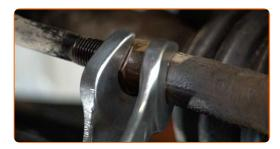
Unscrew the fastening nut connecting the tie rod end to the steering knuckle. Use a drive socket #18. Use a ratchet wrench.
