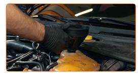
Pour coolant in the coolant reservoir.
