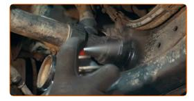
Disconnect the coolant pipe retaining clip.
