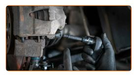
16 Remove the brake caliper.
