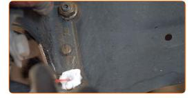
Disconnect the transverse stabilizer fastener from the link. Use a combination spanner #16. Use XZN #6. Use a ratchet wrench.
