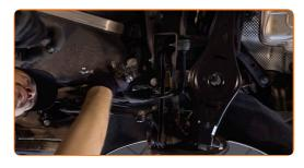
Install a new rod, tighten the fasteners.
