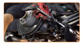
Clean the wheel rim mounting seat. Use a wire brush. Treat the contacting surface. Use copper grease.
