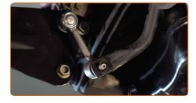
Tighten the fastener connecting the stabilizer link to the stabilizer bar. Use a combination spanner #16. Use XZN #6. Use a torque wrench. Tighten it to 45 nm torque.
