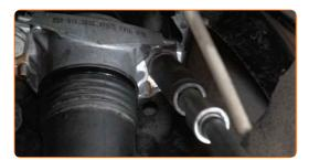
Treat the shock absorber mount fasteners. Use copper grease.
