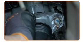
Tighten the shock absorber mount fasteners. Use a drive socket #16. Use a torque wrench. Tighten it to 50 Nm torque.+45°
