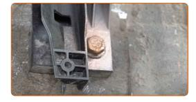
Install the wheel arch cover to its mounting seat.
