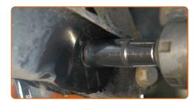
Clean the locker fasteners. Use a wire brush.
