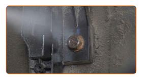
Unscrew the charcoal canister fastener. Use a drive socket #13. Use a ratchet wrench.
