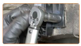
Treat the charcoal canister fastener. Use copper grease.
