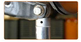
19 Remove the fastening bolt.
