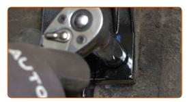
Move the charcoal canister aside to gain access to the upper shock absorber fasteners.
