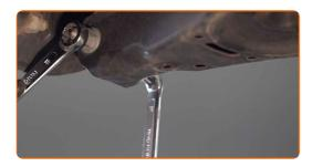
Remove the exhaust system fastener.
