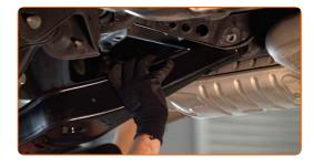
18 Install the control arm fasteners.
