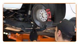
Remove the fastening bolt.
