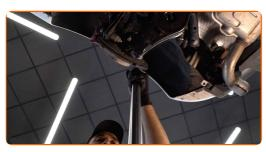
Install the exhaust system fastener.
