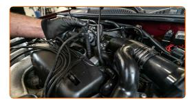
Plug in the connector on the engine intake manifold.
