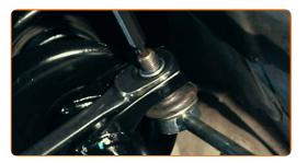
12 Tighten the fastener connecting the stabilizer link to the shock strut. Use a drive socket #19. Use a torque wrench. Tighten it to 65 Nm torque.
