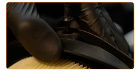
Reinstall the air filter cover. Fasten it.
