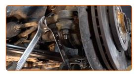
Unscrew the end fastening nut to the steering knuckle. Use a drive socket #17. Use a tap wrench.
