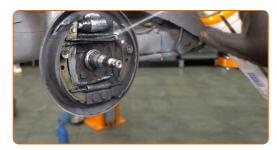
Remove the hold-down spring. Use round-nose pliers.
