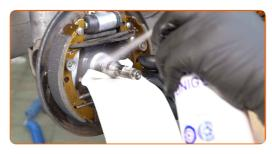
Install the brake drum assembled with the wheel hub bearing.
