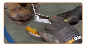
21 Install the brake shoe adjuster lever.
