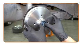
Screw on the hub nut. Use a drive socket #30. Use a ratchet wrench.
