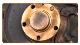
Remove anti-corrosion grease from the new brake disk. Use a brake cleaner.
