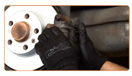
Tighten the brake caliper fasteners. Use a combination spanner #15. Use a drive socket #13. Use a torque wrench. Tighten it to 35 Nm torque.
