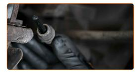
Clean old grease and rust stains, if there are any, from the caliper guide pins and guide pin boots. Use a brake cleaner.
