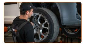
Turn the steering knuckle to the right to get access to the brake hose bolt and brake pad wear sensor.
