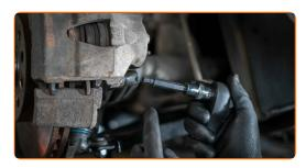
16 Remove the brake caliper.
