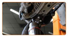
Tighten the ball joint fastener. Use a drive socket #13. Use a torque wrench. Tighten it to 20 Nm torque.+90°
