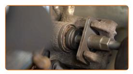
Unscrew the brake disc mounting bolts and remove it. Use Torx T30.
