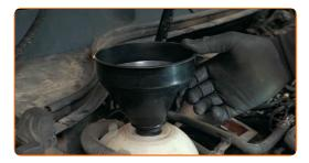
Pour coolant in the coolant reservoir.
