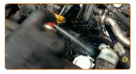
Install the new thermostat housing together with the thermostat.
