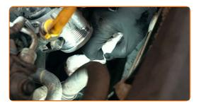
Clean the mounting seat of the air intake hose. Use all-purpose cleaning spray.
