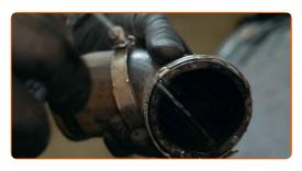
Reinstall the air intake duct.
