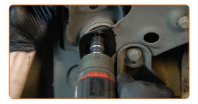
Remove the fastening bolts. Use a drive socket #18.
