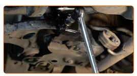
Unscrew the rear fastener connecting the control arm to the subframe. Use a combination spanner #18. Use a drive socket #18. Use a tap wrench.
