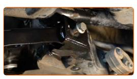
Install the rear fastener of the arm. Use a crowbar.
