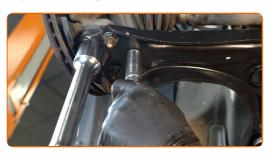
Remove the support from under the arm.
