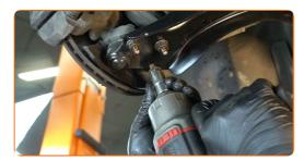
Screw the rear fastener connecting the control arm to the subframe. Use a combination spanner #18. Use a drive socket #18. Use a ratchet wrench.
