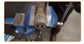
Remove the shock absorber piston rod fastening. Use a combination spanner #17. Use an adjustable wrench.
