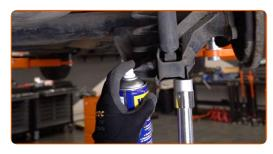
Unscrew the lower fastener of the shock absorber. Use a drive socket #16. Use a combination spanner #16. Use a ratchet wrench.
