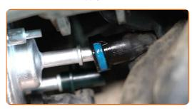
Screw in the fuel filter mounting bracket. Use a Phillips screwdriver.
