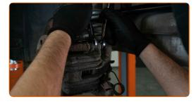
11 Remove the brake caliper.
