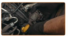
56 Tighten the throttle body fasteners to the air intake manifold. Use Torx T27. Use a torque wrench. Tighten it to 14 nm torque.
