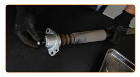
Tighten the shock absorber mount fasteners. Use a combination spanner #16. Use an adjustable wrench. Use a torque wrench. Tighten it to 25 Nm torque.
