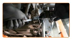
Unscrew the upper fastener of the shock absorber. Use a drive socket #16.
