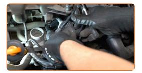
Replacement: ignition coil – AUDI A1 Hatchback (8X1, 8XK). AUTODOC recommends:
