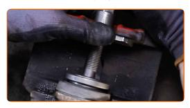
18 Install the brake caliper guide pins.
