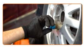
Lower the car and working in a cross order, tighten the wheel bolts. Use a torque wrench. Tighten it to 120 Nm torque.
