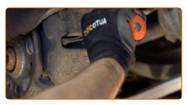
10 Remove the brake caliper.
