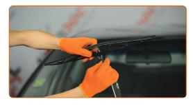
Remove the blade from the wiper arm.
