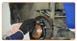
Screw the brake cylinder fastening bolts. Use Torx T30. Use a torque wrench. Tighten it to 8 nm torque.
