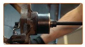
Remove the bearing inner race from the wheel hub. Use a bearing separator. Use 3-Arm Gear Puller.
