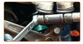
Install and tighten the drive shaft bolt. Use HEX No.H14.
