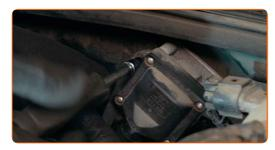
A Remove the ignition coil.
