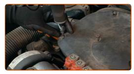
Remove the air filter housing.
