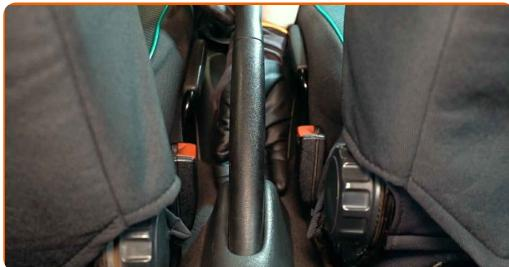
**2** Loosen the parking brake cable. Use a combination spanner #10.
