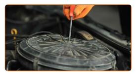
Release the air filter cover clips.
