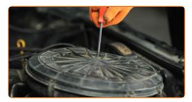
Release the air filter cover clips.
