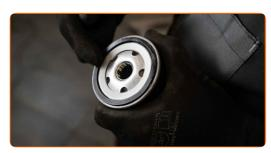
Screw the new filter into its place. Use the 76/14-F socket. Observe the recommended tightening torque.
