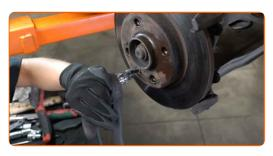
15 Remove the brake disc.
