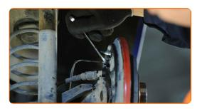
Bleed the brake cylinder system. Use a combination spanner #7.
