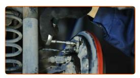
Remove the brake cylinder from the backplate. Use a flat screwdriver.
